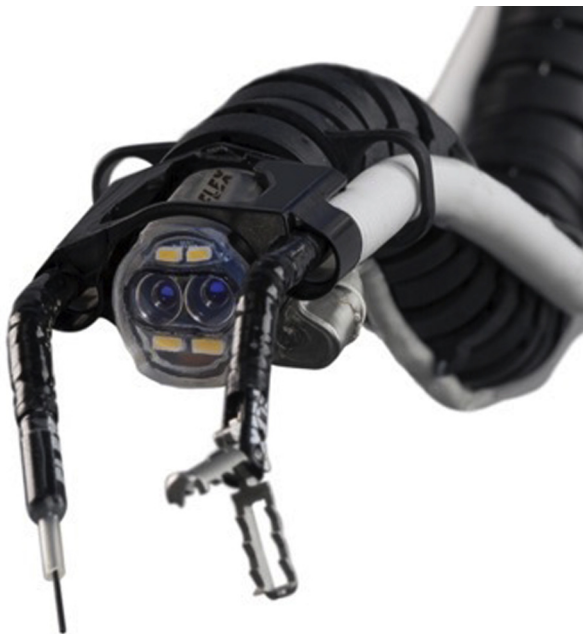
Figure 1. The robot's flexible distal end including 2 working channels with a needle-knife and grasper (image used with permission from Medrobotics, Raynham, Mass, USA).
